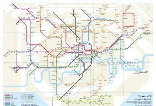
That clay is good for tunnelling is evident when looking at the tube map. There are only few tunnels south of the Thames as there are only few clay deposits. The clay was an abundant material resource with large availability.
